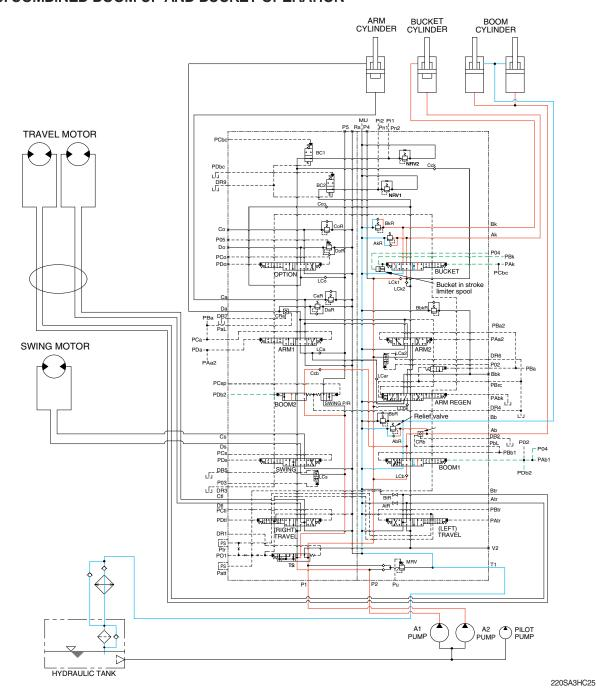
When the boom up and bucket functions are operated, simultaneously each spool in the main control valve is moved to the functional position by the pilot oil pressure (PAb1, PDb2, PAk, PBk) from the remote control valve.
