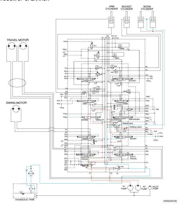
When the right control lever is pulled back, the boom spools in the main control valve are moved to the up position by the pilot oil pressure (PAb1, PDb2) from the remote control valve.
